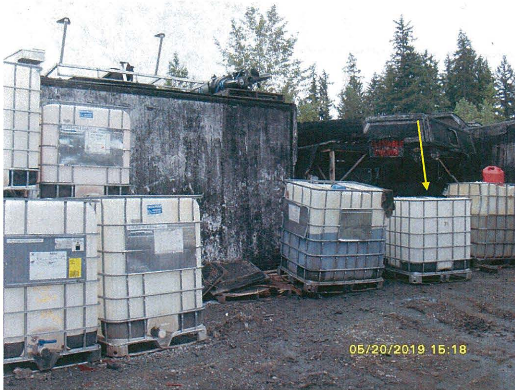
Photo 6 (SI850999): Nine totes stored uncovered and without secondary containment. According to facility representatives, the 6 totes on the left of the photo were empty and the 3 totes on the right contained motor oil (left tote), an unknown petroleum chemical (center tote identified by a yellow arrow) which was leaking onto the ground, and gasoline (right tote).
