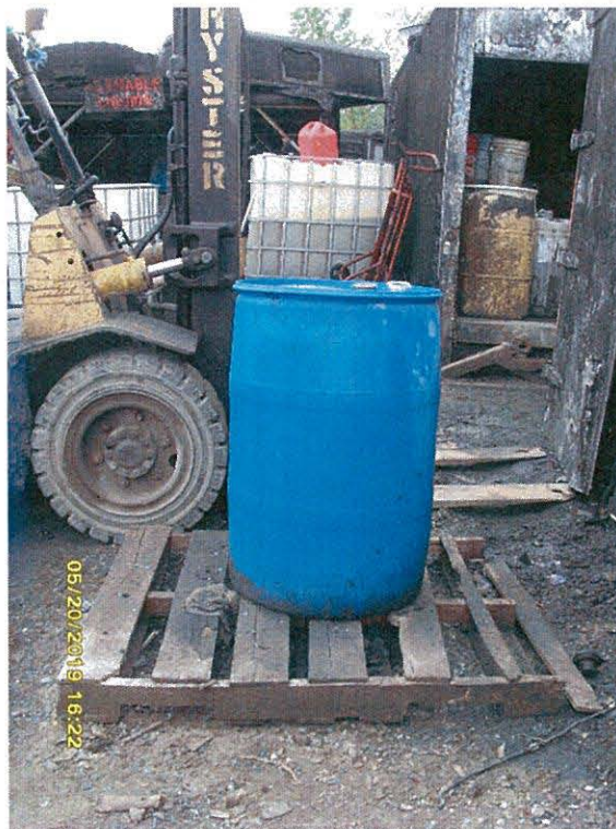
Photo 8 (SI851030): An empty barrel stored uncovered and without secondary containment on the southwest side of the main building.
