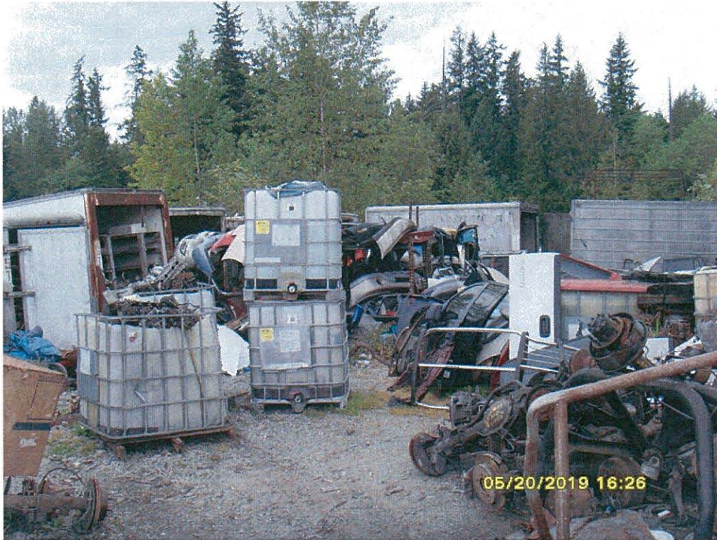
Photo 27 (SI851034): Western view of 2 totes stored uncovered and without secondary containment south of the main building. According to the tote labels, they contained transmission fluid.
