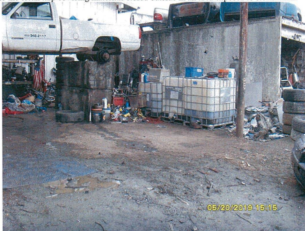
Photo 5 (SI850997): Three totes stored without secondary containment in the vehicle fluid draining area on the back side of the main building. According to facility representatives, they contained anti-freeze, motor oil, gear lube, and transmission oil.
