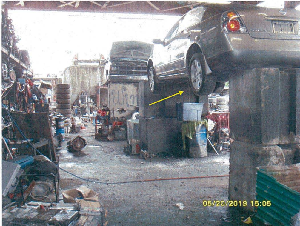
Photo 3 (SI850990): Vehicle fluid draining area under cover on the back side of the main building. Note the fluid draining from the car in the foreground into a plastic bin (yellow arrow) and the granular absorbent below the car.
